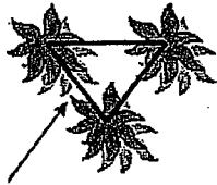
Example: shrubs planted thirty-six inches (36") on center, with triangular spacing.
